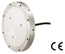
The KDJ-PA and KDK-PA are stainless-steel soil pressure gauges each 200 mm in outside diameter. They are load-cell-type soil pressure gauges and designed with a high level of resistance to lateral pressure. The difference between these two models is the way the cable is attached to the gauge body.
