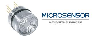
MPM280TH pressure sensor has similar outline, installation dimension and sealing methods as general MPM280 pressure sensor. For construction material, the isolated diagram uses tantalum material and housing uses Hastelloy C material. The sensor is sealed by FKM O-ring. It can be used to measure strongly corrosive media. The pressure range is -1.0bar~0bar~1.0bar...350bar.
